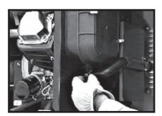
Finally, insert the plastic plug that came with the generator into the hole on the bottom of the air cleaner base.
